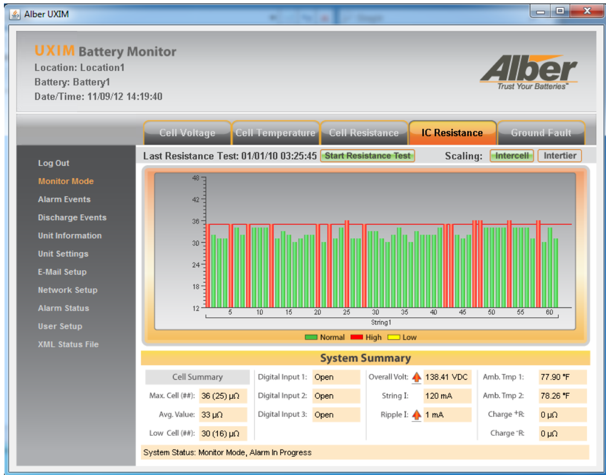
Figure 8 – Intercell Resistance Readings and Summary Information
