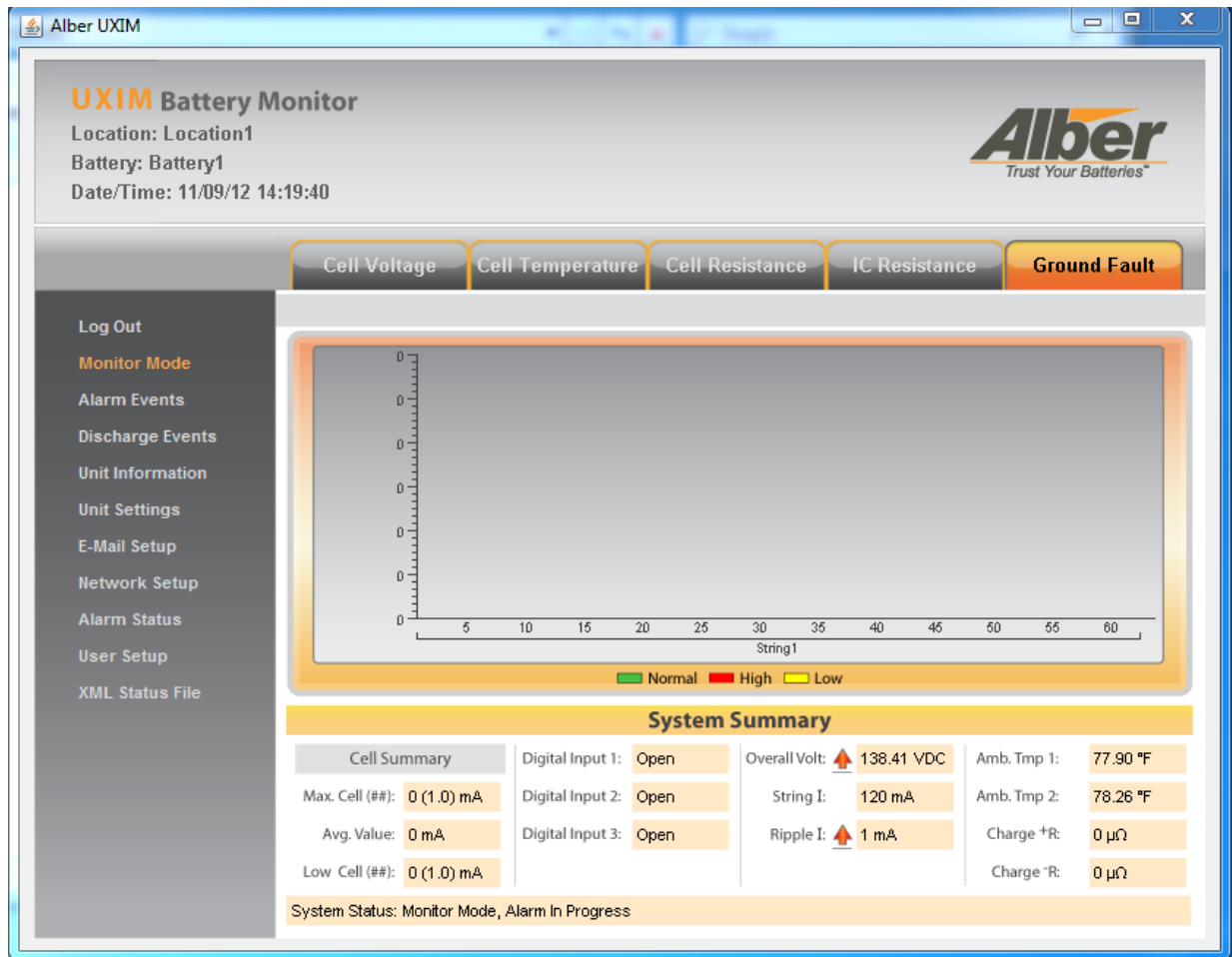
Figure 9 – Ground Fault Readings and Summary Information
