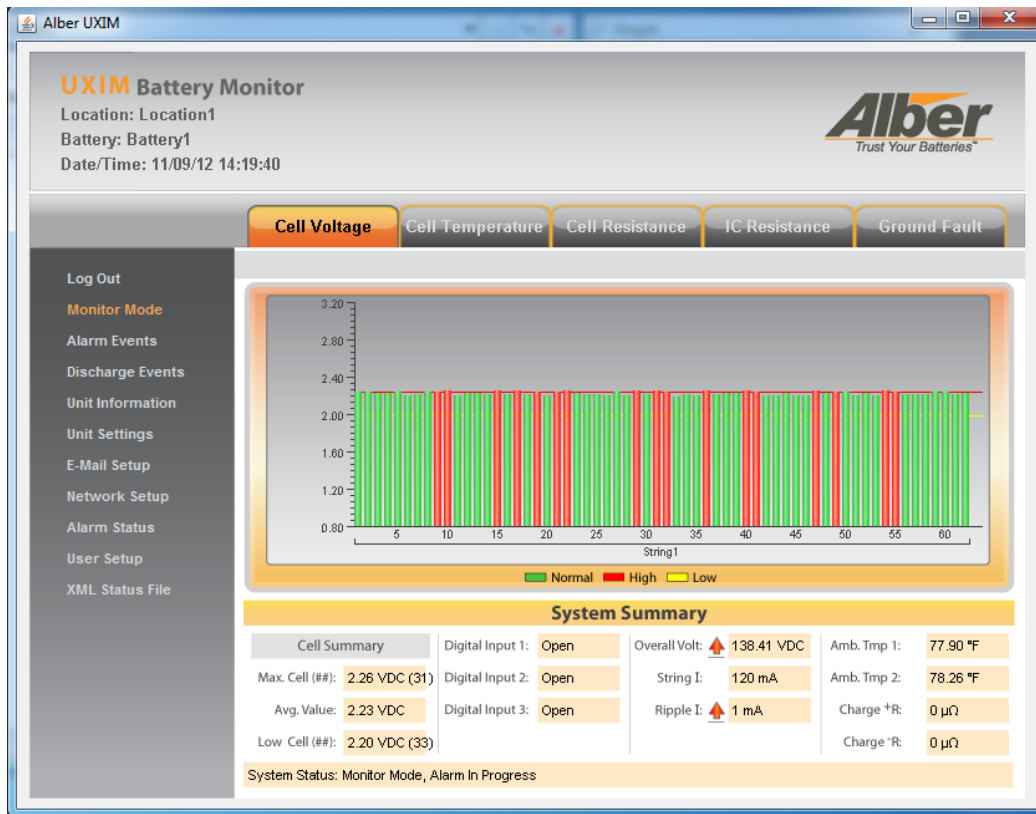
Figure 5 – Cell Voltage Readings and Summary Information
